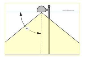
*Fully shielded luminaire* means a fixture constructed and installed in such a manner that all light emitted by it, either directly from the lamp (bulb) or a diffusing element, or indirectly by reflection or refraction from any part of the fixture, is projected below the horizontal. This can be determined by a "field test" or visual assessment of an operating sample, or fixture photographs and/or diagrams.
