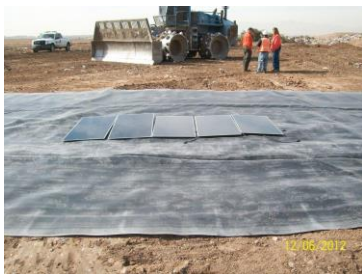
Fig. 5. Aljon model 91K compactor used to crush PV modules in a Municipal Solid Waste Landfill in the State of Arizona, USA.
