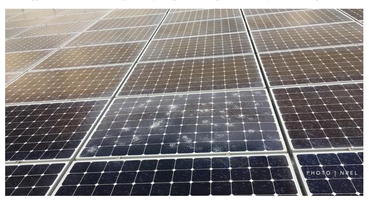
$<sup>\</sup>hfill \Box$  Just one PV panel out of more than 3,000 was damaged at NREL following the hailstorm. Photo | NREL PV Strong
