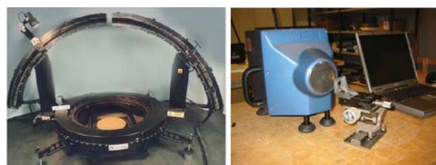
FIGURE 2 | Left: Goniometer used for albedo measurements. Right: Instrument used for emissivity measurements.
