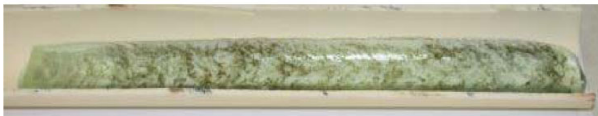
Figure 4. (a) Sample after being heated up to 900°C for 1 h; (b) after being heated up to 1000°C for 2 h; (c) after being heated up to 1100°C for 3 h
