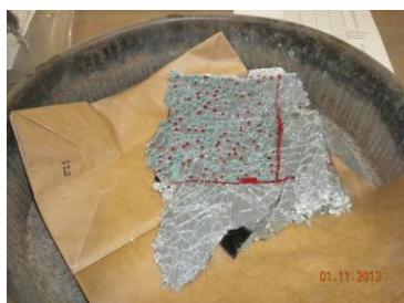
Fig. 6. Compactor foot punch-out of a PV module crushed in a Municipal Solid Waste Landfill in the State of Arizona, USA.
