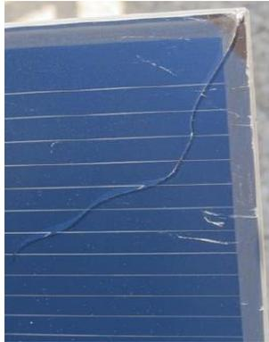
Module breakage is rare and occurs only in approximately 1% of modules over 25 years or 0.04% per year. More than one-third of breakages occur during shipping and installation, therefore the broken modules are removed prior to plant operation. During operation, most breakages consist of impact fractures in which the module is still bound together by the industrial laminate.
