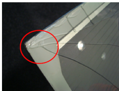
Figure 19 Example of typical breakage pattern of First Solar modules
