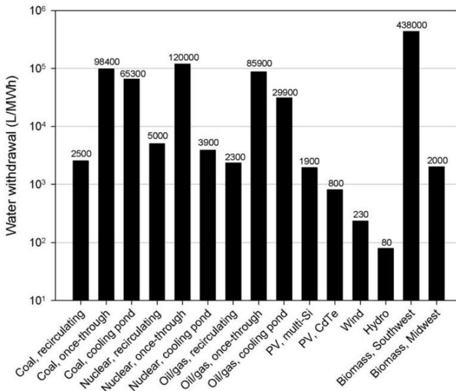
**Figure 47** Life-cycle water withdrawal of electricity generation technologies<sup>177</sup>. Assumptions for CdTe PV are  $\eta = 10.9\%$ ,  $T = 30$  yr,  $PR = 0.8$  and  $Irr = 1,800$  kWh/(m<sup>2</sup>·yr).
