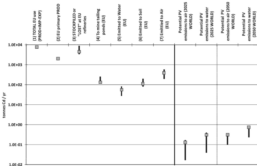
**Figure 44** Current Cd flows in EU-27 compared to potential future global Cd emissions caused by CdTe PV (logarithmic scale)<sup>153</sup>. Assumed maximum cumulative capacities are 260 GW<sub>p</sub> in 2025 and 1 TW<sub>p</sub> in 2050.
