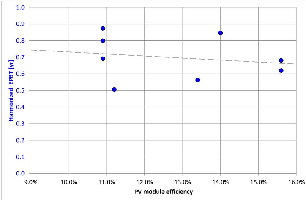
**Figure 36** Energy Pay-Back Time (EPBT) of ground-mounted CdTe PV systems, vs. increasing PV module efficiency; all values harmonized to  $T = 30$  yr,  $PR = 0.8$ ,  $Irr = 1,700$  kWh/(m<sup>2</sup>·yr) and  $\eta_e = 0.31$  (data from Table 8).
