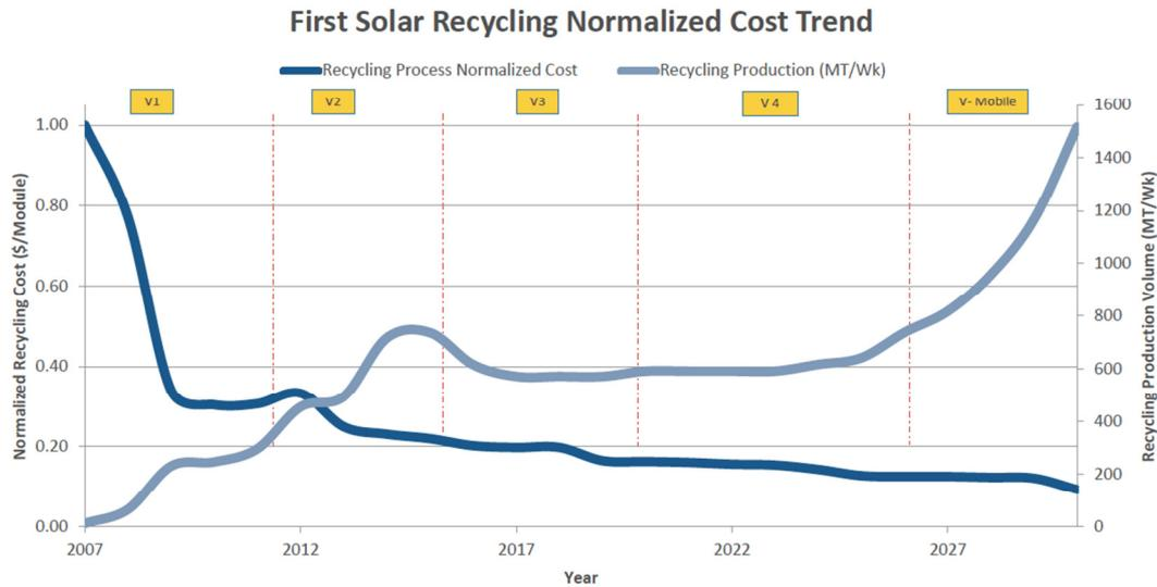
Figure 23: Evolution of the normalized recycling costs (US\$/module) for First Solar CdTe PV module recycling process. Version V2 is currently in place, with V3 expected to come in line shortly.
