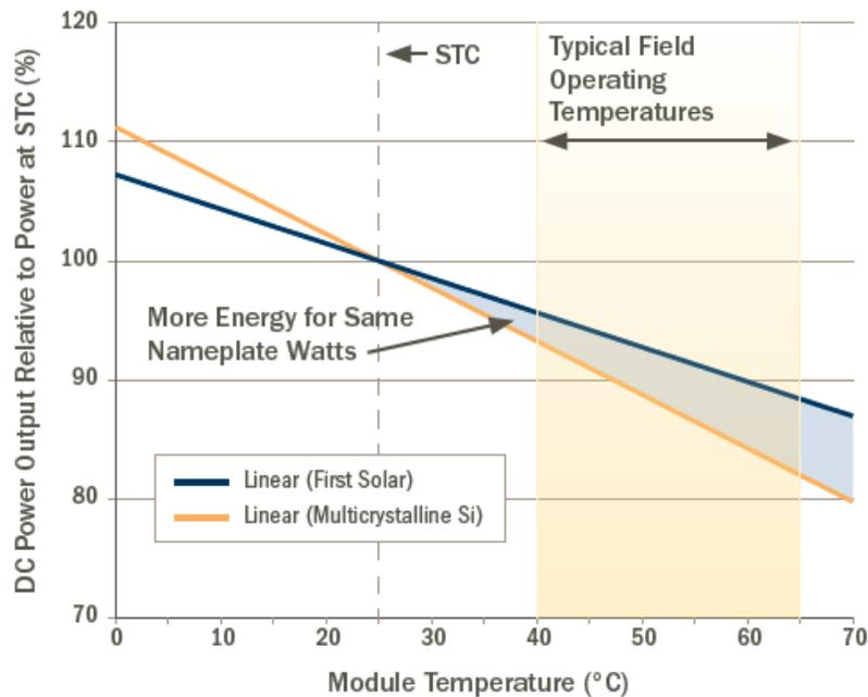
**Figure 18** Comparison between the temperature dependence of CdTe modules with respect to multicrystalline silicon. First Solar’s Series 4 and 4A temperature behavior (blue line) and standard multi c-Si modules (orange line) versus module output power (First Solar Series 4 data sheet) modules<sup>37</sup>.
