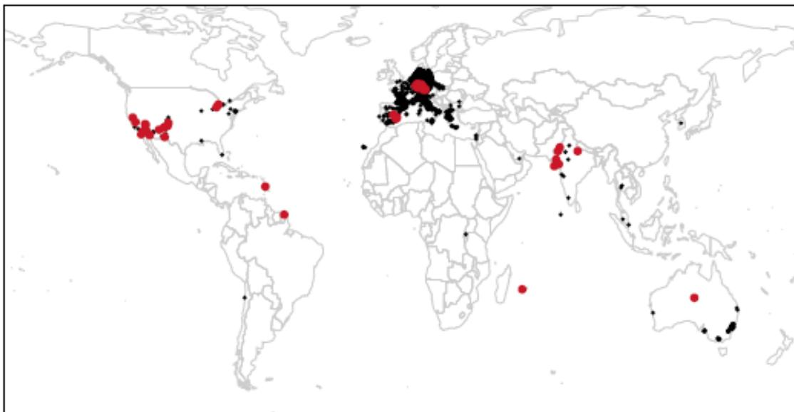
**Figure 15** Location of First Solar power plants (black dot) and field reliability monitored sites (red dot)<sup>19</sup>.
