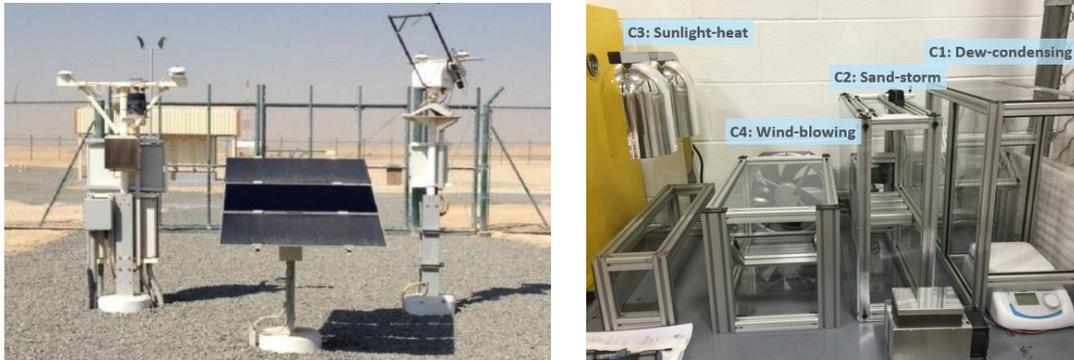
**Figure 26** (left) Soiling monitoring station at test site in UAE. (right) Lab scale environmental simulator for anti-reflective coating development<sup>59</sup>.
