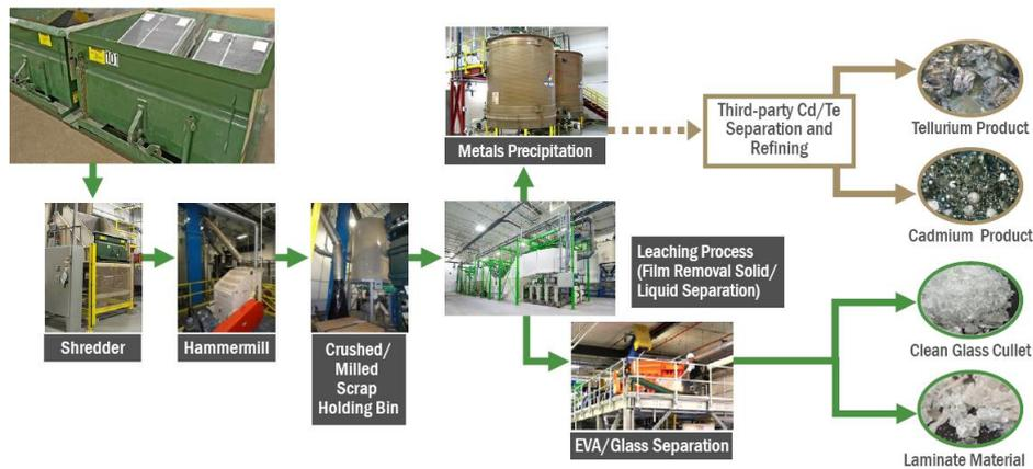
Figure 32 Flow chart of CdTe PV module recycling process<sup>78</sup>.
