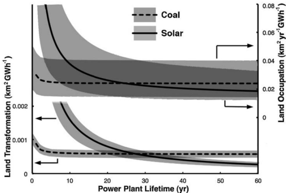
**Figure 46** Land transformation and land occupation for PV and coal-fired electricity<sup>174</sup>. Assumptions for PV are  $\eta = 13\%$ ,  $PR = 0.8$ ,  $I_{rr} = 1,700 \text{ kWh}/(\text{m}^2 \cdot \text{yr})$ .
