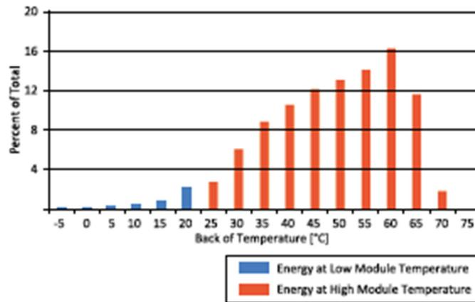
Figure 30: Distribution of the fraction of power production as a function of back-of-module temperatures for a First Solar PV power plant operating in the USA desert Southwest area [58].
