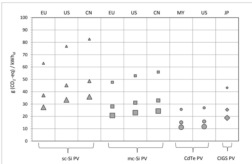
**Figure 38** Global Warming Potential (GWP) of ground-mounted PV systems under three different irradiation levels<sup>146</sup>. Small symbols: 1,000 kWh/(m<sup>2</sup>-yr); medium symbols: 1,700 kWh/(m<sup>2</sup>-yr); large symbols: 2,300 kWh/(m<sup>2</sup>-yr). EU= European Union; US= United States of America; CN= China; MY= Malaysia; JP= Japan.
