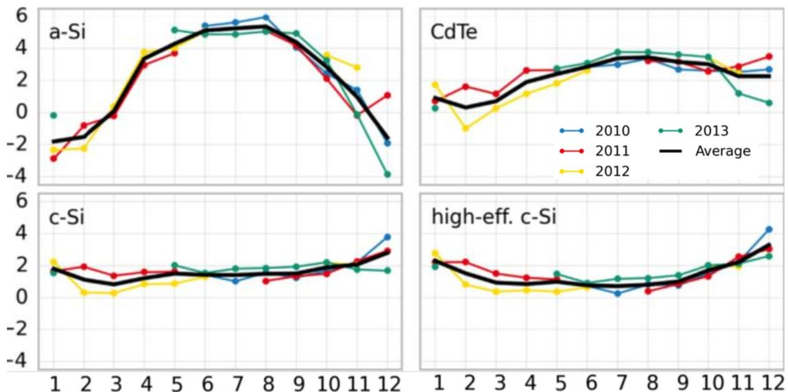
Figure 24 Monthly Spectral impact of PV technologies over 3 years measurements made in Freiburg (Germany)<sup>45</sup>.
