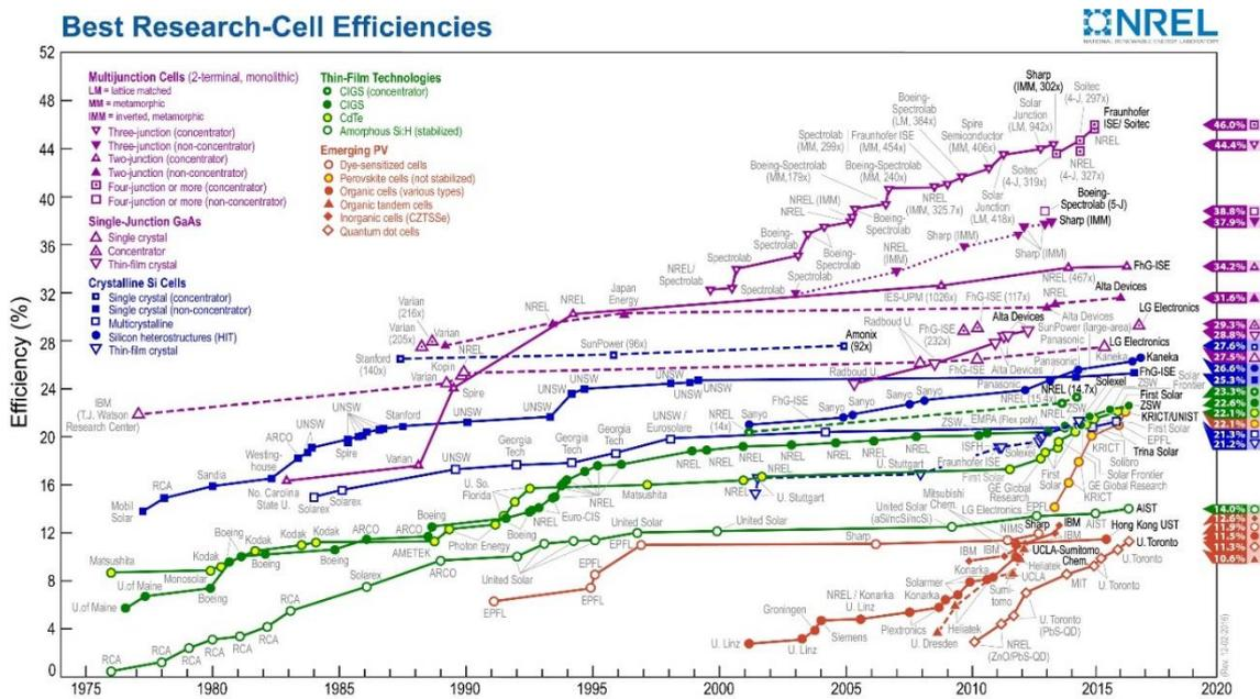
Figure 1 Record efficiencies of PV Solar cells (from NREL as of 17<sup>th</sup> December 2016).
