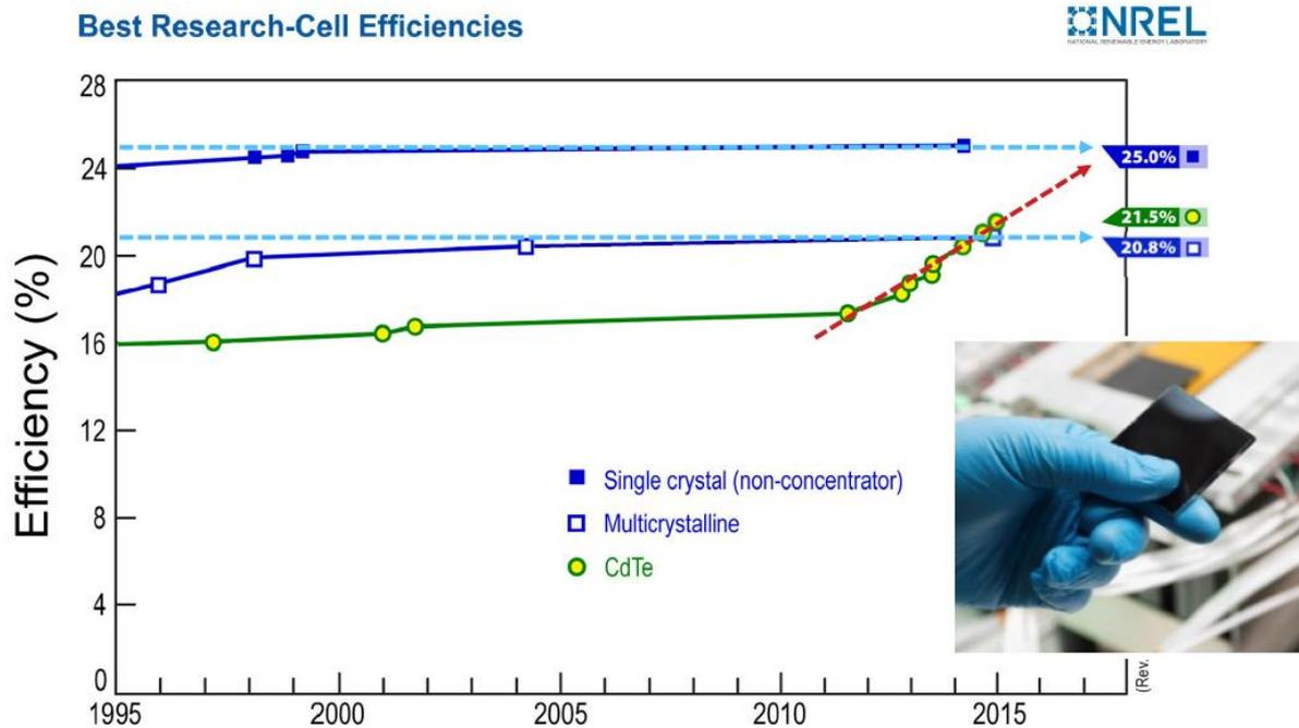
Figure 3. The National Renewable Energy Laboratory's solar cell efficiency chart showing the evolution of the single crystal, multi-crystalline and CdTe technologies
