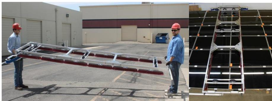
**Figure 27** Manual Dry Brush Trolley designed for First Solar modules from Aztera<sup>62</sup>.
