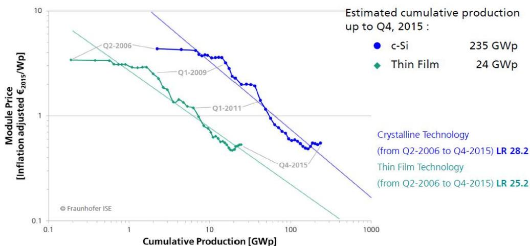
**Figure 10** Learning curves for the prices of PV modules comparing CdTe technology (mainly First Solar) and c-Si technology<sup>15</sup>.
