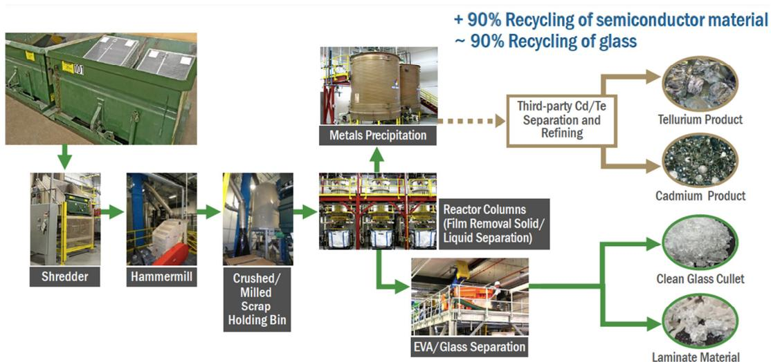
Figure 22: Process flow of First Solar’s CdTe PV module recycling process. After metal precipitation carried out in-house, Cd and Te separation and refining are done by third parties.
