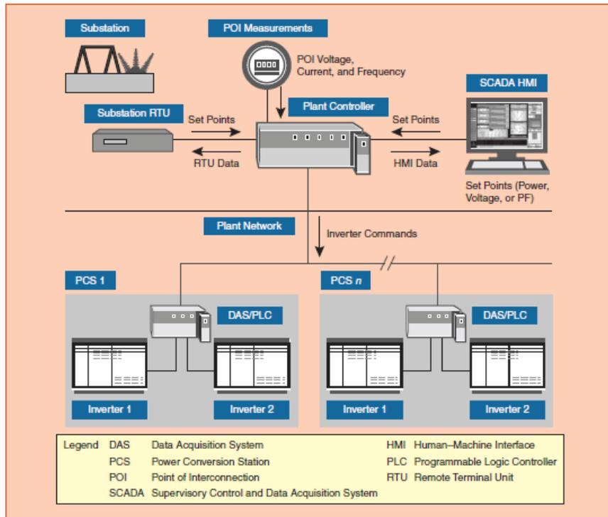
Figure 28 Example of a plant control system and interfaces to other components<sup>68</sup>.
