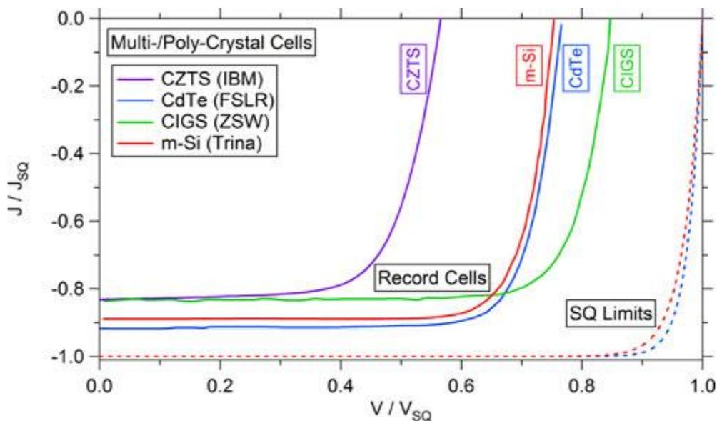
**Figure 3** Comparison of the I-V curves of record cell technologies (CIGS, CdTe and m-Si) with the ideal Shockley Queisser limit<sup>9</sup>.
