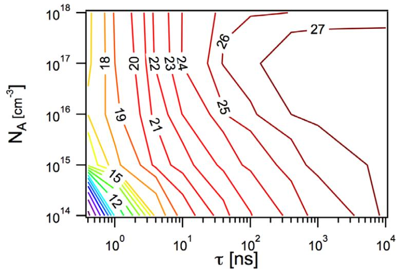
**Figure 5** Simulated contour plots of conversion efficiencies of CdTe solar cells versus bulk life time and acceptor doping level<sup>7</sup>.
