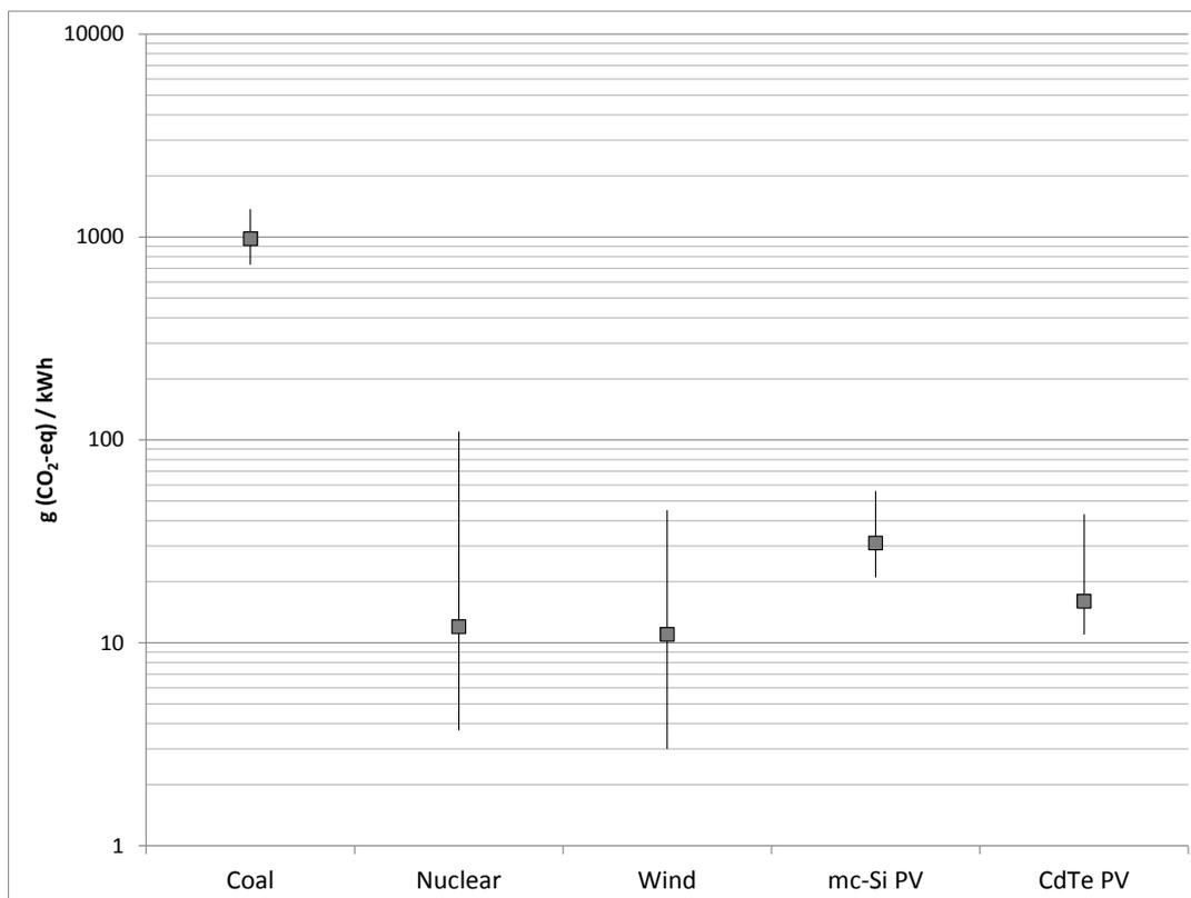
**Figure 42** Minimum, maximum and median harmonized literature values for Global Warming Potential (**GWP**) of coal-fired, nuclear, and wind electricity, compared to latest values for mc-Si PV and CdTe PV electricity<sup>146</sup>, respectively for  $I_{rr} = 1,000 \text{ kWh}/(\text{m}^2\cdot\text{yr})$ ,  $I_{rr} = 2,300 \text{ kWh}/(\text{m}^2\cdot\text{yr})$  and  $I_{rr} = 1,700 \text{ kWh}/(\text{m}^2\cdot\text{yr})$ .
