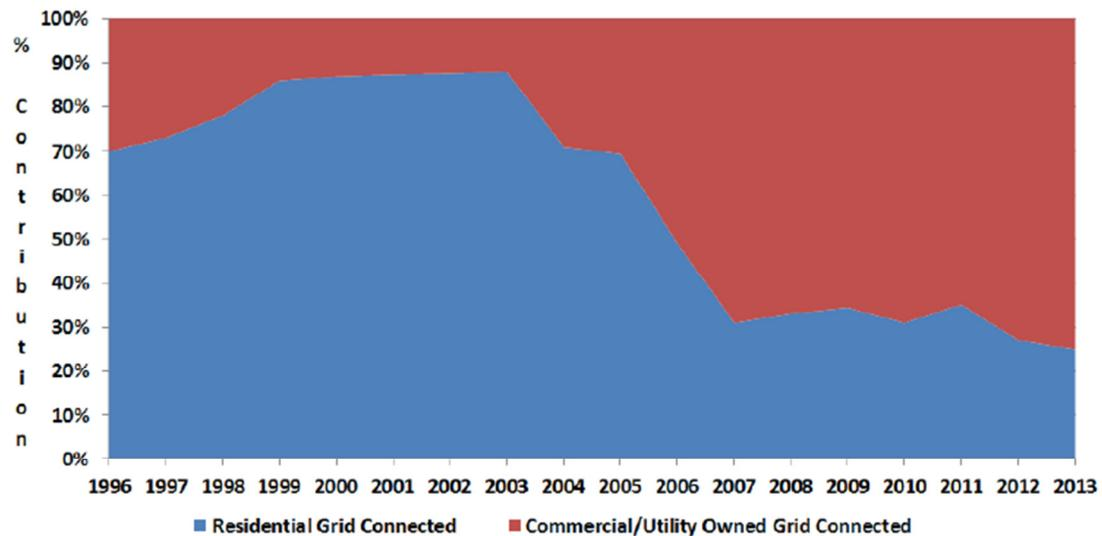
Figure 10: Evolution of the share between small-scale, residential grid-connected and utility-scale, multi-megawatt solar PV installations [39]. Large-scale currently represent more than 2/3 of the world PV market.
