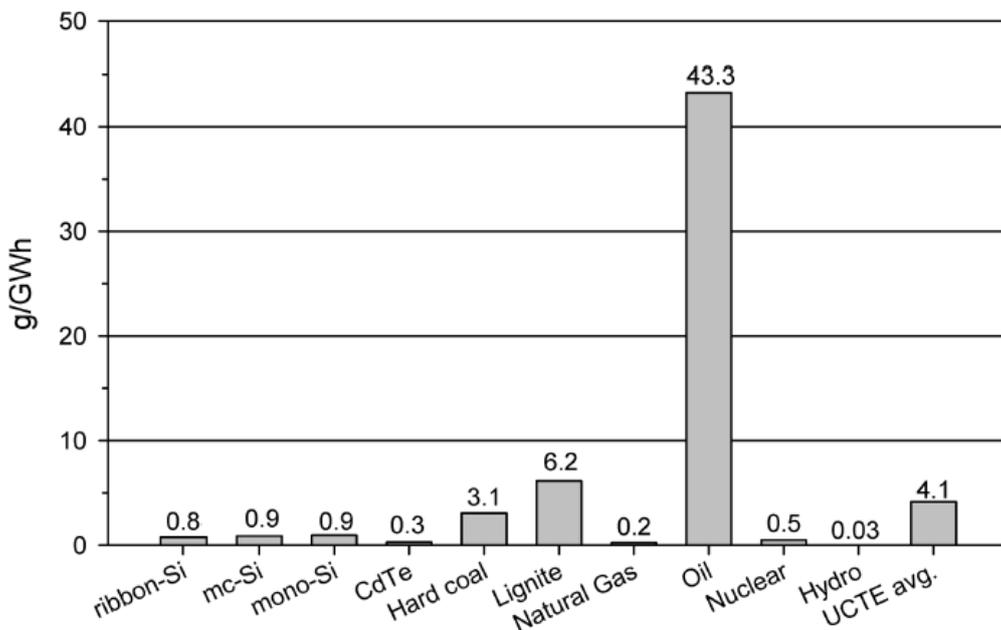
**Figure 43** Life-cycle Cd emissions of electricity generation technologies<sup>159</sup>. Assumptions for CdTe PV are  $\eta = 9\%$ ,  $T = 30$  yr,  $PR = 0.8$  and  $Irr = 1,700$  kWh/(m<sup>2</sup>-yr).
