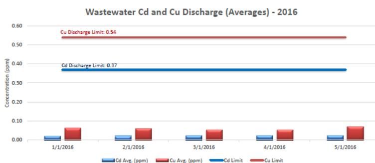
**Figure 33** Wastewater Cd and Cu concentration<sup>78</sup>.
