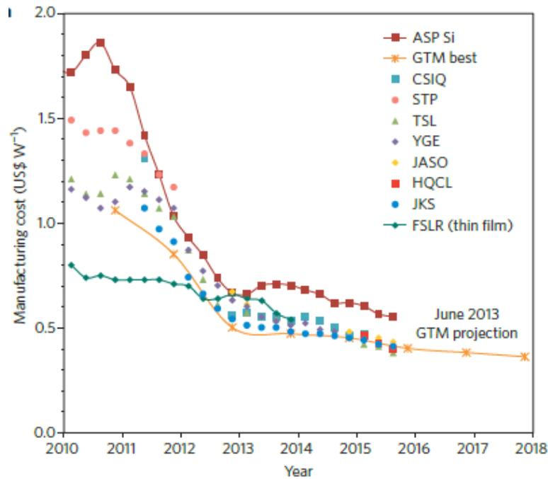
**Figure 12** Evolution of module manufacturing costs presented as a function of the c-Si suppliers and for a thin film manufacturer (First Solar)<sup>13</sup>.
