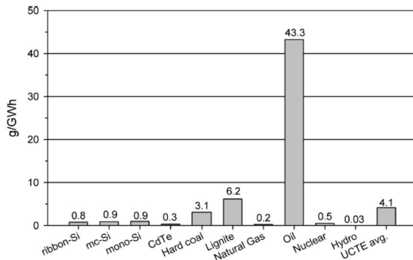
**Figure 8. Life cycle atmospheric Cd emissions for PV systems from electricity and fuel consumption, normalised for a Southern Europe average insolation of 1 700 kWh/m<sup>2</sup>/yr, performance ratio of 0.8, and lifetime of 30 yrs (Fthenakis, et al., 2008).**
