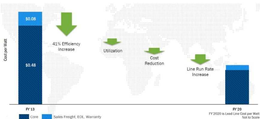
**Figure 13** First Solar's module cost reduction until 2020.
