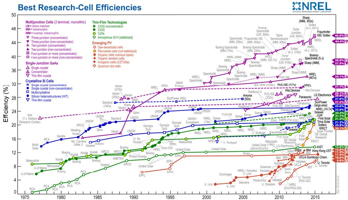
Figure 1: The National Renewable Energy Laboratory – NREL’s solar cell efficiency chart [29] showing the evolution of the best research-cell efficiencies since the 1970’s (updated June 2015).
