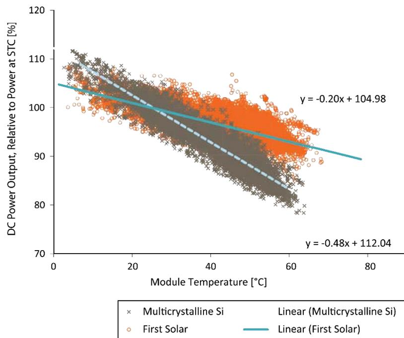
Figure 5. First Solar and multi-crystalline DC power output vs temperature (Strevel, et al., 2012)
