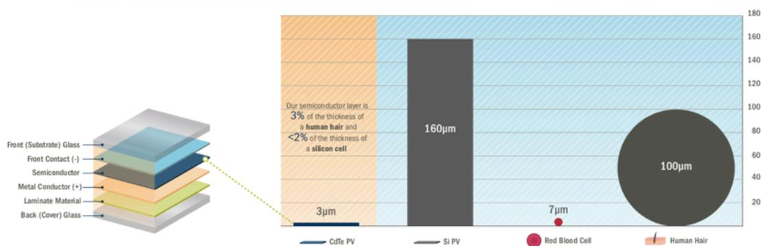
Figure 2: A CdTe photovoltaic system (top), and a schematic cross-section of a CdTe photovoltaic module (bottom). For comparison, the central CdTe layer is thinner than the thickness of the corresponding semiconductor layer in a silicon photovoltaic device, or the diameter of a red blood cell, or the thickness of human hair. Image source: First Solar, Inc.
