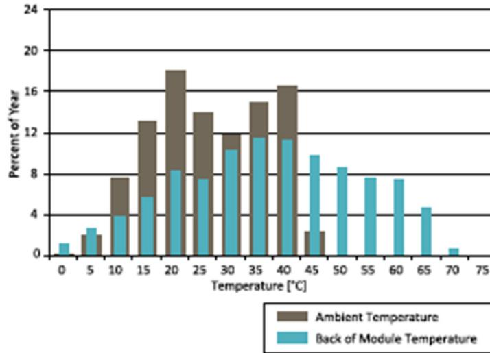
Figure 29: Distribution of ambient and back-of-module surface temperatures measured in a First Solar PV array in the USA desert Southwest area [58].
