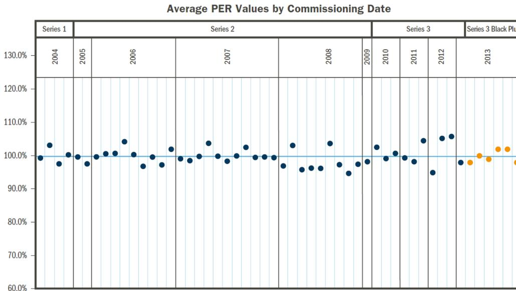
**Figure 17** Average Predicted Energy Ratio (PER) by commissioning year for 270 MW of thin-film CdTe PV systems using First Solar modules: >270 MW monitored installations base, including >130 MW of hot-climate deployments<sup>34</sup>. Orange dots highlight the performance of the production series (S3 black plus) with included ZnTe back contact.
