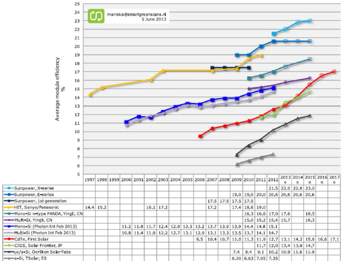
Figure 6 Historical roadmap average (real and estimated) total area module efficiency of commercial PV modules<sup>12</sup>.
