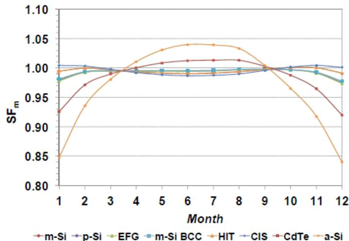
**Figure 23** Modeled data of the spectral factor for the different technologies in Stuttgart<sup>42</sup>.
