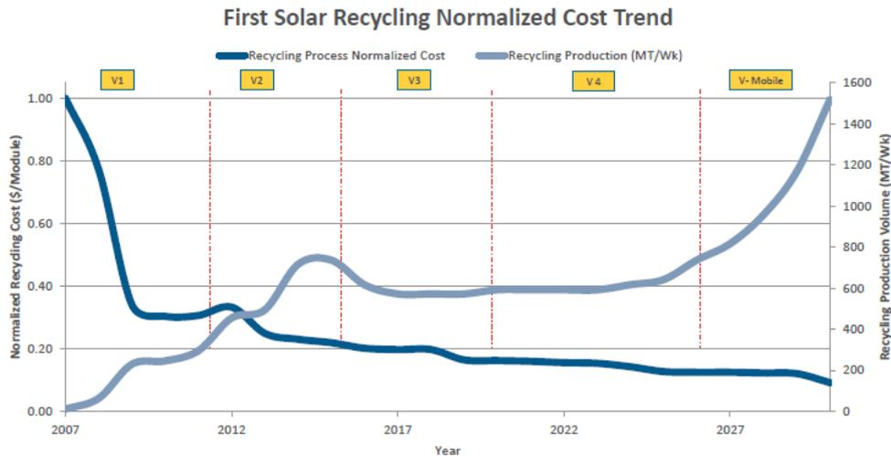
**Figure 34** First Solar’s recycling normalized cost trend<sup>113</sup>.
