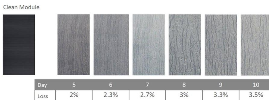
**Figure 25** Field images of soiling accumulation on FS modules at DEWA site (Dubai, UAE)<sup>55</sup>.
