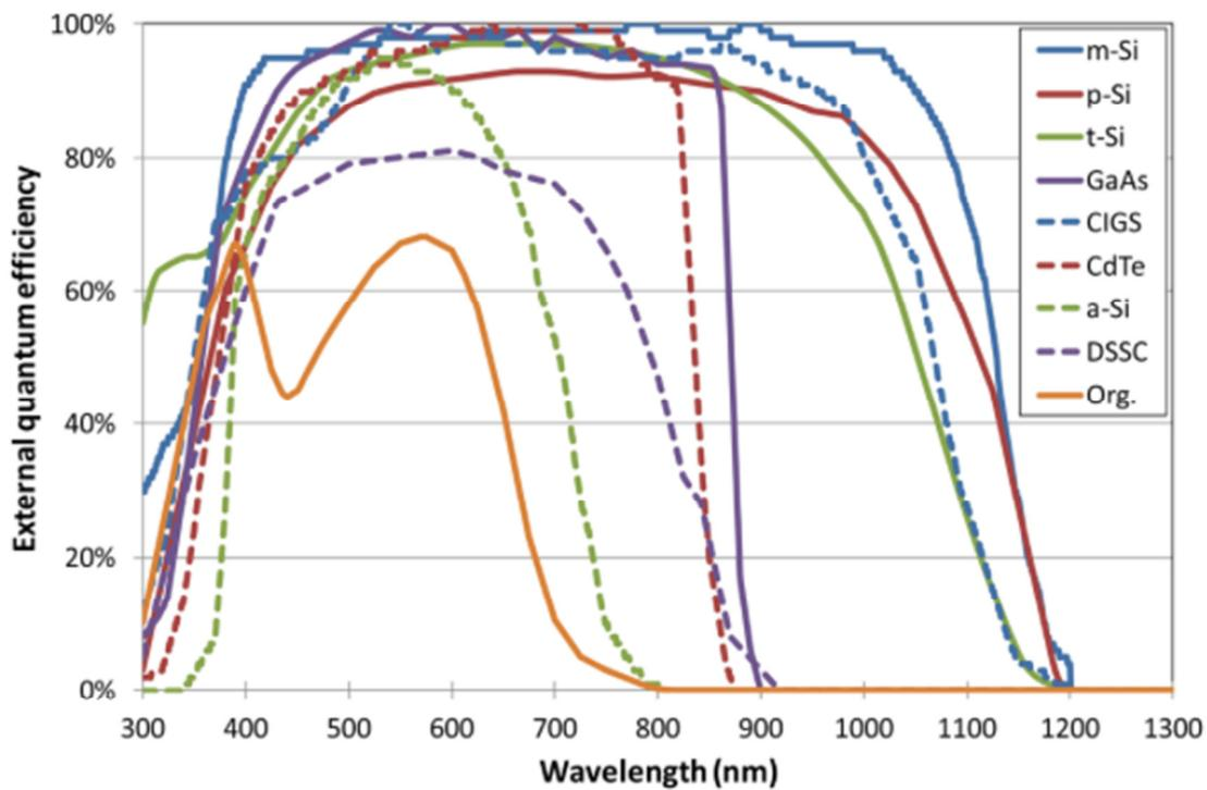
Figure 7: External quantum efficiency curves for a number of solar cell materials. The more shifted to the left (lower wavelengths) a curve is, the better the corresponding material will respond to a blue-shifted spectral content of light [37].
