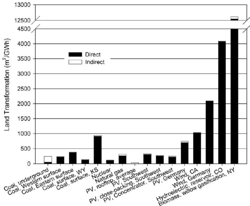
**Figure 45** Land transformation for a range of electricity generation technologies<sup>173</sup>. Assumptions for PV are  $\eta = 13\%$ ,  $T = 30$  yr,  $PR = 0.8$ ,  $Irr = 1,800$  kWh/(m<sup>2</sup>-yr) for “rooftop, average”, and  $Irr = 2,400$  kWh/(m<sup>2</sup>-yr) for “Southwest”.
