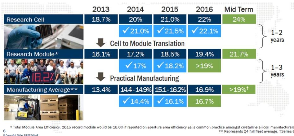
**Figure 9** Technological roadmap of First Solar from cells results objectives to module objectives<sup>14</sup>.
