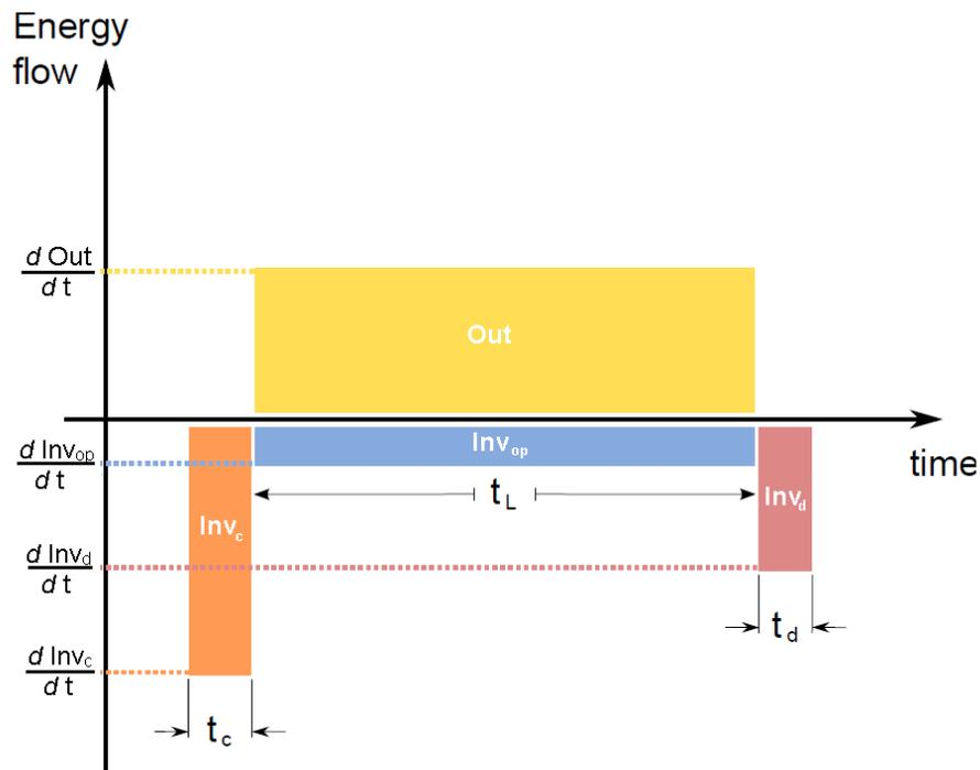
**Figure 35** Schematic depiction of the energy ‘investments’ ( $Inv_c + Inv_{op} + Inv_d$ ) and of the energy ‘return’ (**Out**) of a PV system. The individual areas are drawn for illustrative purposes only, and are not intended to be quantitatively representative of a typical CdTe PV system. Source: Raugai *et al.*<sup>122</sup>, adapted from Herendeen<sup>123</sup>.
