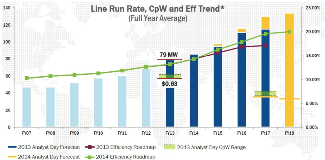
Figure 12: Annual increments in First Solar Line Run Rates, and the reviewed Efficiency Roadmap, with PV module efficiencies of 15% at the end of 2014, 20% in 2017-18.
