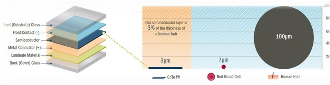
**Figure 31** Schematic representation of First Solar's module architecture<sup>76</sup>.
