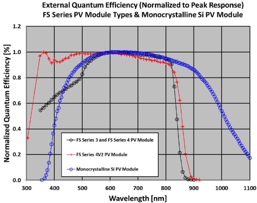
**Figure 16** Normalized external quantum efficiency of First Solar FS Series 3, FS Series 4 and FS Series 4V2 CdTe PV module types compared with that of a single-crystalline Si PV module<sup>23</sup>. The specific properties of CdTe outdoor performance can be directly derived from its characteristic spectral response at short wavelengths (< 500 nm).
