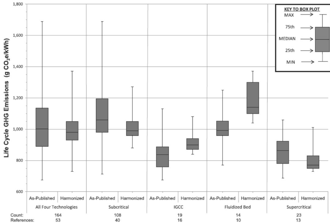
**Figure 39** Global Warming Potential (GWP) of coal-fired electricity<sup>150</sup>.
