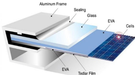
Figure 2: Components of crystalline silicon panels. The vast majority of silicon panels consist of a glass sheet on the topside with an aluminum frame providing structural support. Image Source: [www.riteksolar.com.tw](http://www.riteksolar.com.tw)
