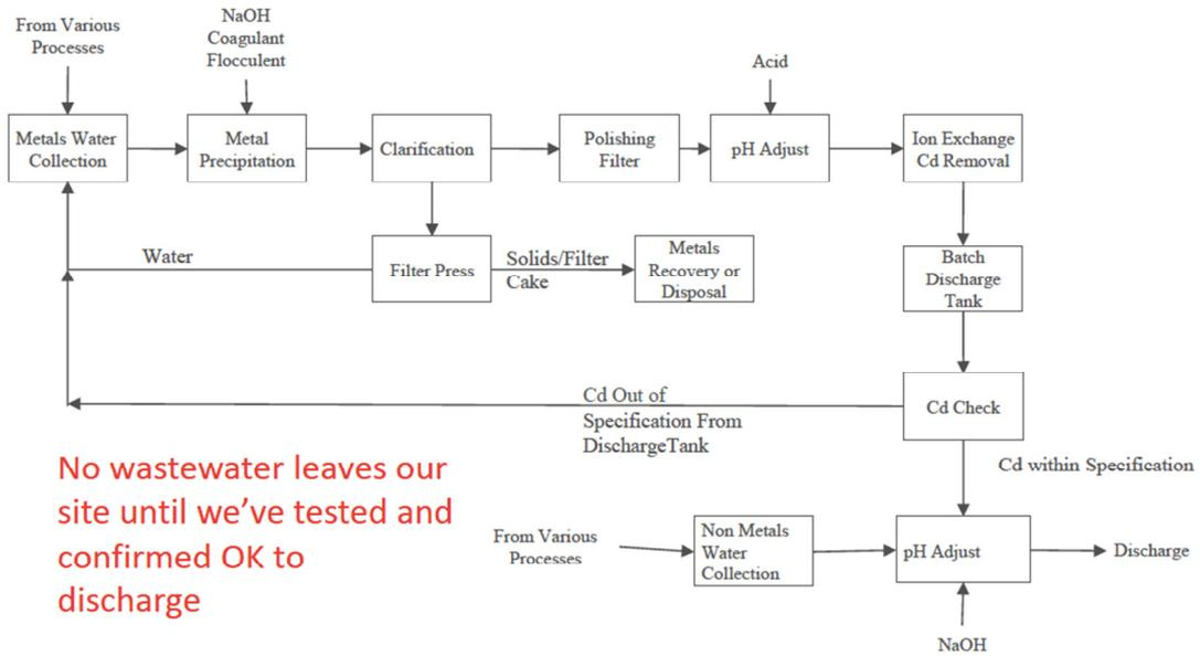
Figure 27: Process flow diagram of the wastewater treatment at First Solar manufacturing plants.
