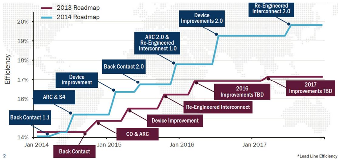
Figure 13: First Solar efficiency roadmap, showing the company's R&D strategies for CdTe PV module efficiency improvements in the period 2014-17.
