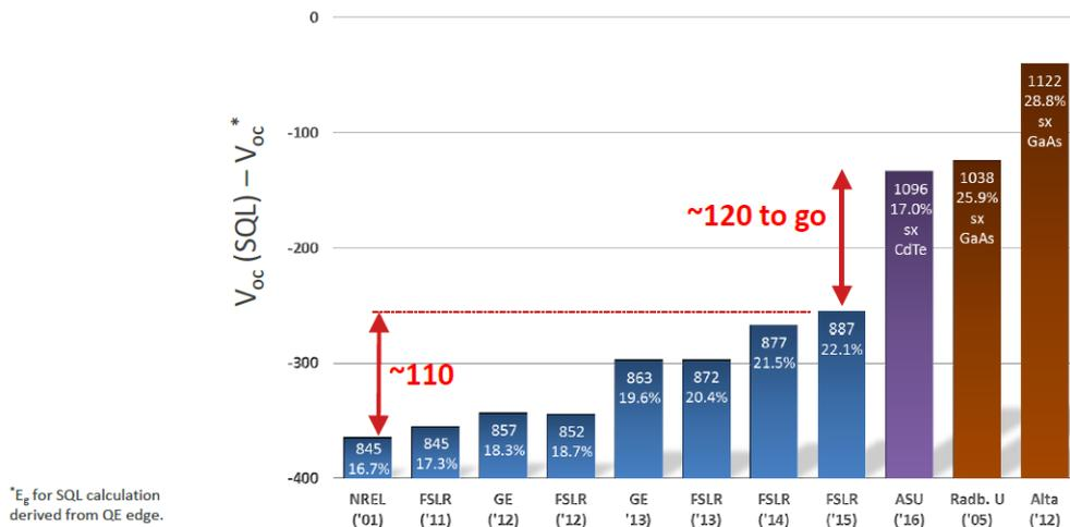
**Figure 4** Roadmap for open circuit voltage improvement in CdTe solar cells, expressed in mV and compared to reference devices, single crystal CdTe and GaAs devices. The Y value corresponds to the difference between the calculated theoretical open circuit voltage from the band gap value and that of the real device<sup>2</sup>.
