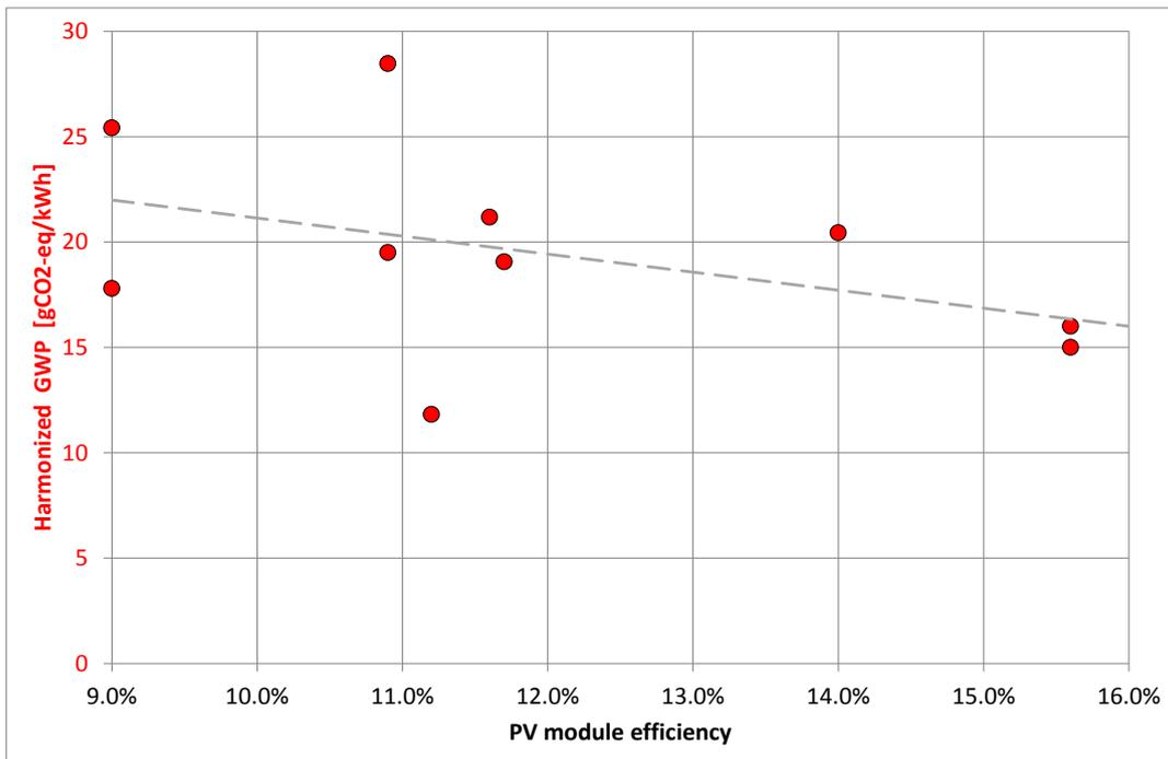
**Figure 37** Global Warming Potential (GWP) for ground-mounted CdTe PV systems, vs. increasing PV module efficiency; all values harmonized to  $T = 30$  yr,  $PR = 0.8$ ,  $Irr = 1,700$  kWh/(m<sup>2</sup>·yr) and  $\eta_e = 0.31$  (data from Table 8).
