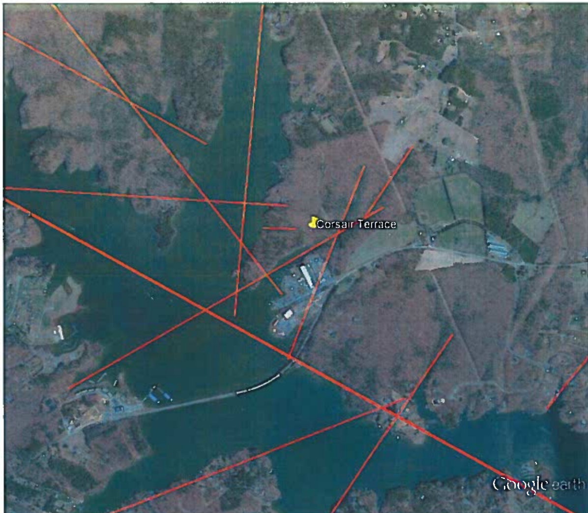
Figure 4 Site Fracture Pattern
